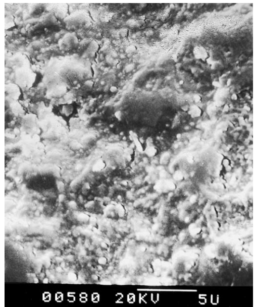
Fig. 15. Morphology of SiC/Cu FGM surface after in situ plasma irradiation.
