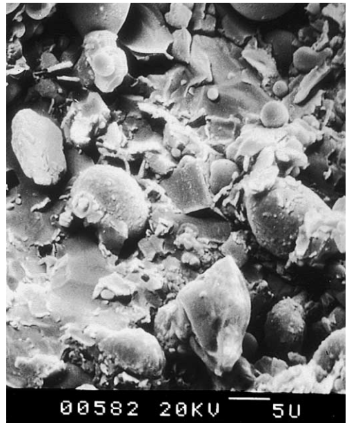
Fig. 14. Morphology of 80 vol.% SiC-contained surface of SiC/Cu FGM after in situ plasma irradiation.
