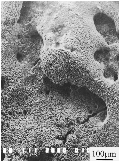
Fig. 11. Ceramic surface of p = 1.0 SiC/Cu FGM after 300 times cyclic hot impact by laser pulse.
