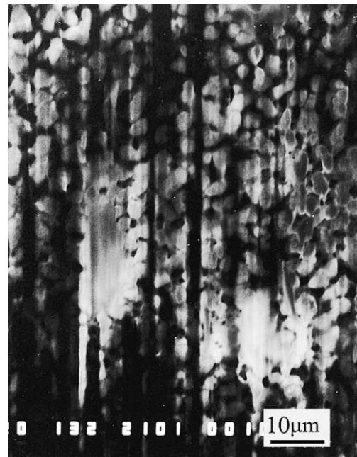
Fig. 13. Microstructure of SiC ceramic layer on the edge of beam spot.
